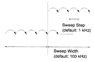
**NOTE:** Sweep width is the frequency width to sweep on both sides of the selected frequency.
